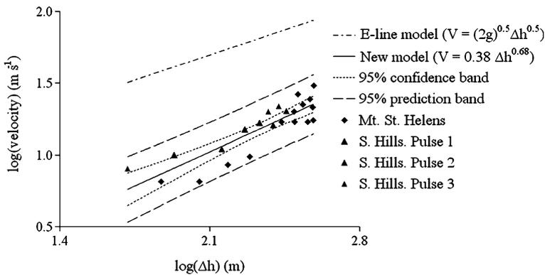
**Fig. 3** Empirical relationship between the vertical distance between the energy line and the surface ( $\Delta h$ ) and the flow velocity (New model), 95% confidence and prediction limits, and both the observed and e-line velocities corresponding to the same  $\Delta h$ , where measurements were carried out
