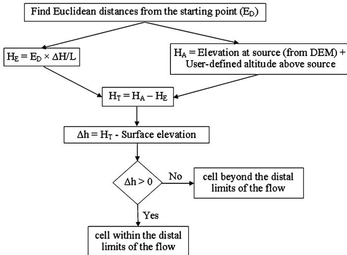
**Fig. 5** Flow diagram describing the principal algorithm used to define the energy cone. If the cell is within the distal limits of the current, then the cell has a value of 1, otherwise it has a value of 0. For the graphic representation of the parameters please refer to Fig. 1
