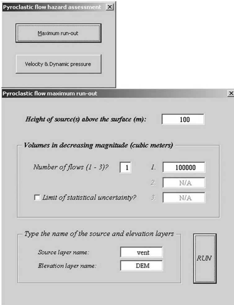
**Fig. 4** Graphic-user interface for the inputs to simulate PDC maximum potential run-out
