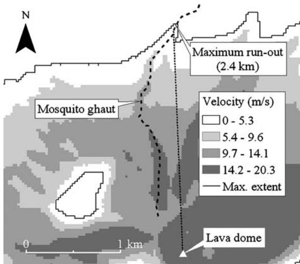
**Fig. 10** Sample output of the velocity ( $\text{m s}^{-1}$ ) of the PDC of 17 June 1997 that travelled 3.0 km down Mosquito Ghaut at Soufrière Hills volcano, Montserrat (West Indies). The inputs, assumptions and digital topography employed are the same as those used for the run shown by Fig. 6
